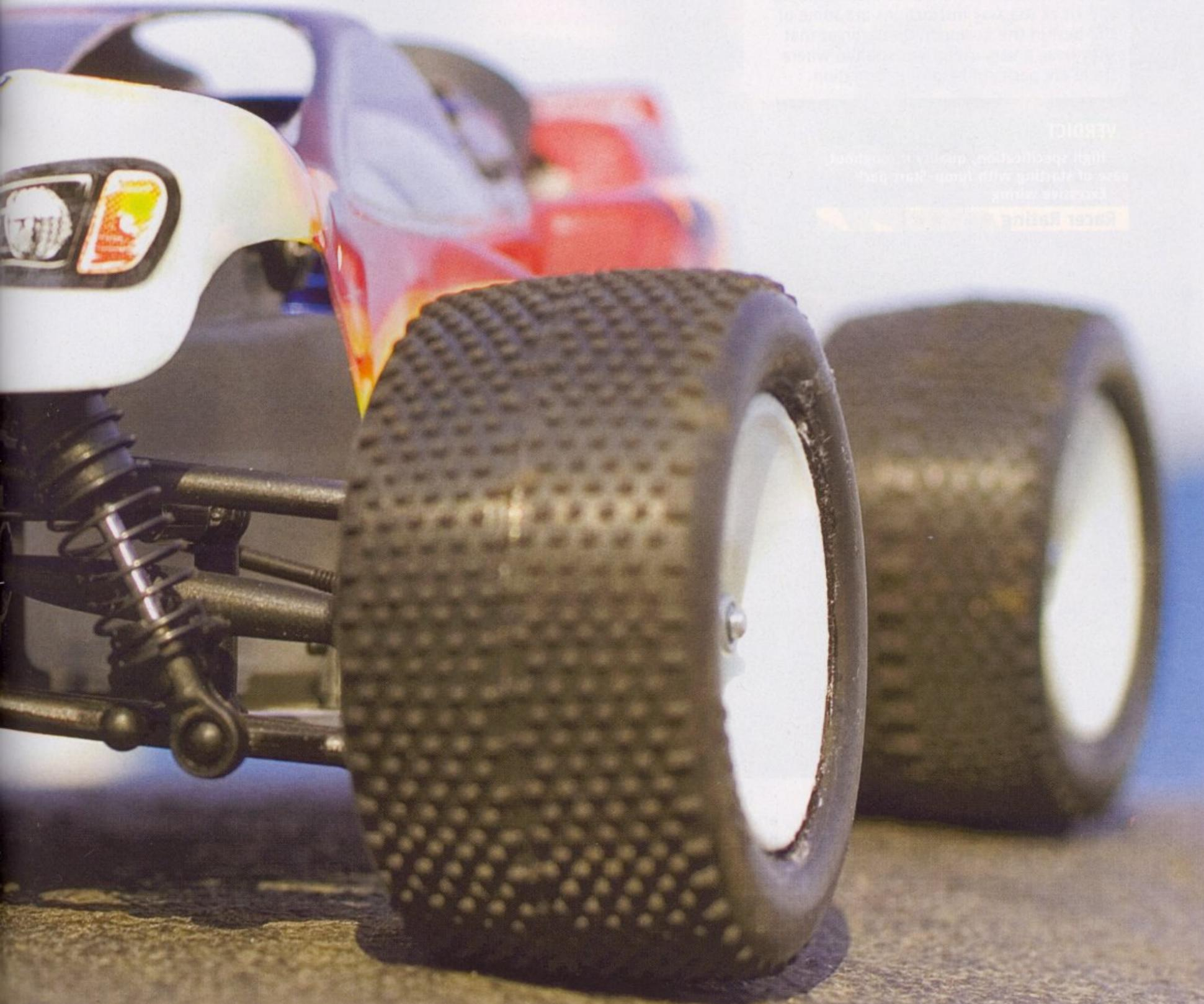
steering blocks. Both the front and rear ends are very similarly made from nylon and composite materials, which can be later updated with aluminium versions available for those keen on adding that extra 'bling'. A combination of steel spur gear, aluminium main driveshaft and ball bearings throughout provide efficient drive to this fierce little truck.
