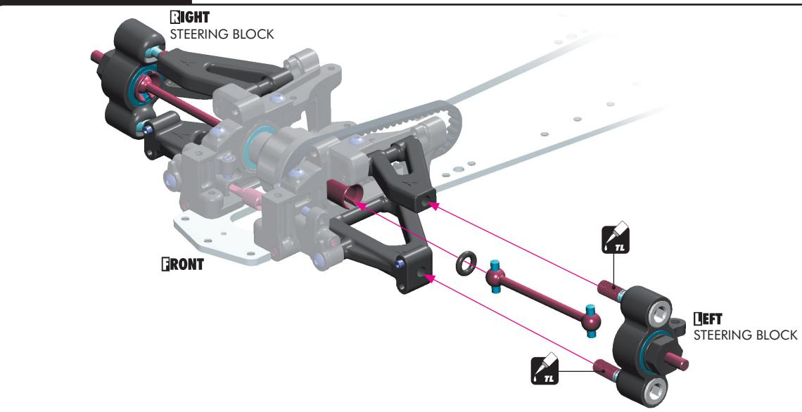
To ensure that the pivot balls do not loosen, you may apply a very small amount of medium (blue) threadlock to the outside threads of the pivot balls. This will help to secure it in the steering block.
