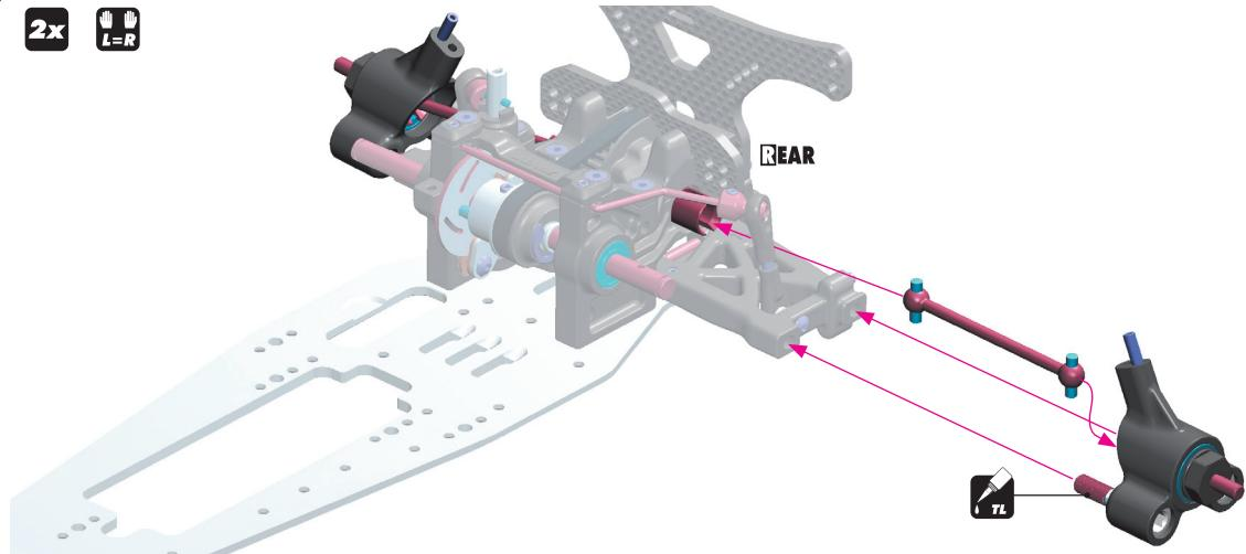
To ensure that the pivot balls do not loosen, you may apply a very small amount of medium (blue) threadlock to the outside threads of the pivot balls. This will help to secure it in the arm.
