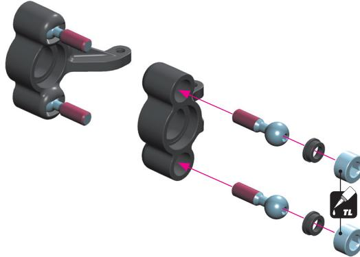
To ensure that the alum nuts do not loosen, you may apply a very small amount of medium (blue) threadlock to the outside threads of the nut. This will help to secure it in the steering block.
