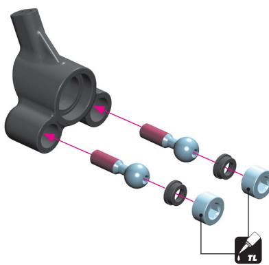
To ensure that the alum nuts do not loosen, you may apply a very small amount of medium (blue) threadlock to the outside threads of the nut. This will help to secure it in the hub.
