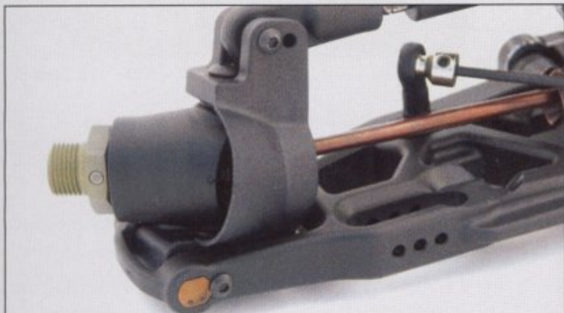
Plastic knuckles decrease the un-sprung weight and the C-hubs feature steel bushings moulded in for extra strength
