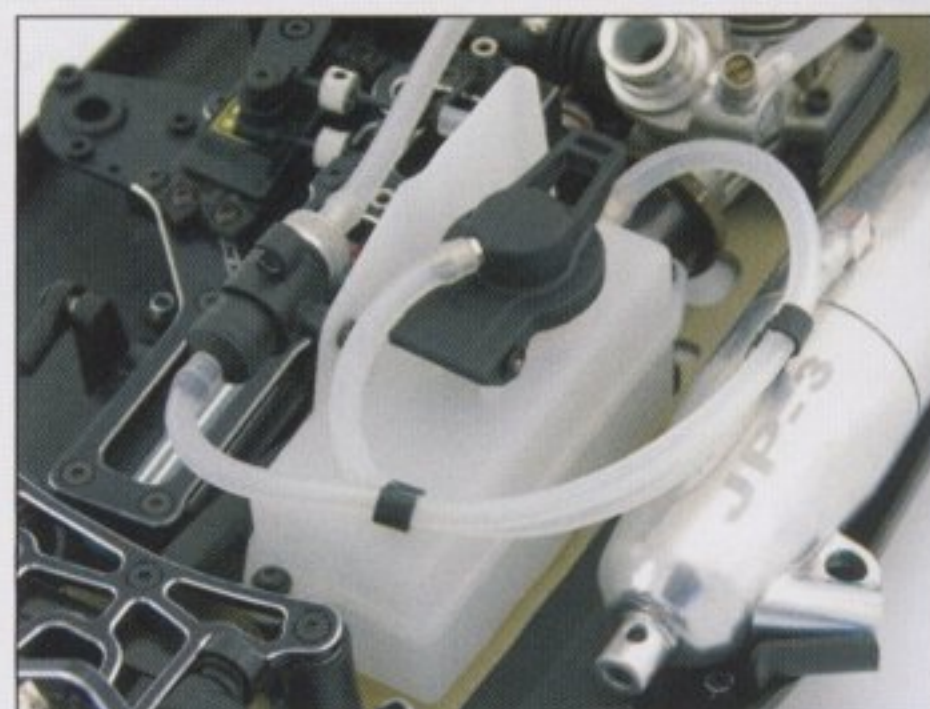
The fuel filter now attaches to the side of the 125cc fuel tank which reduces vibrations as it's mounted on rubber grommets
