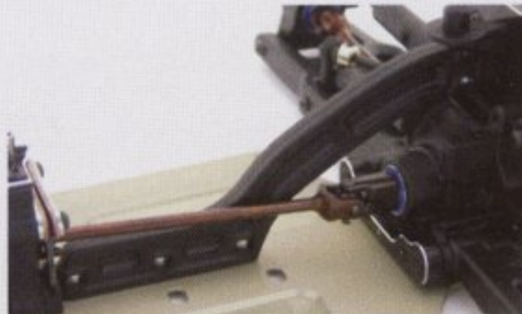
HUDY spring steel CVDs are used throughout and the composite rear brace is firmly attached with three nyloc nuts
