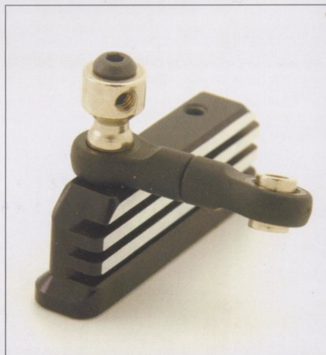
A top tip to get ball ends in is to use something like the engine mount and screw them in
