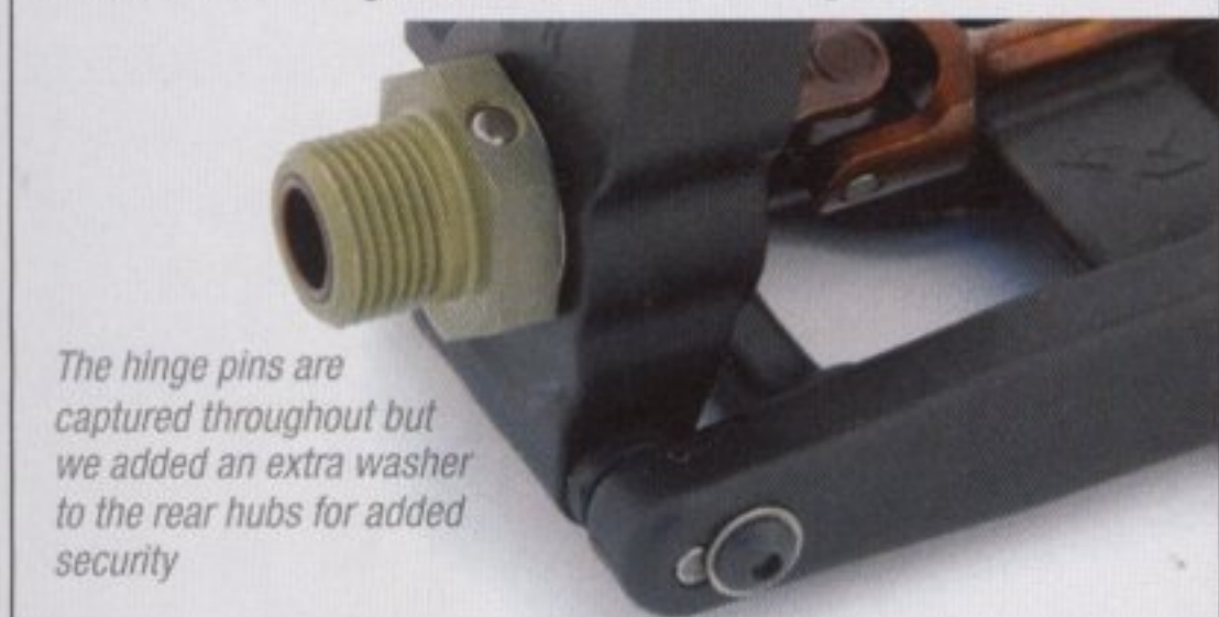
Plastic knuckles decrease the un-sprung weight and the C-hubs feature steel bushings moulded in for extra strength
