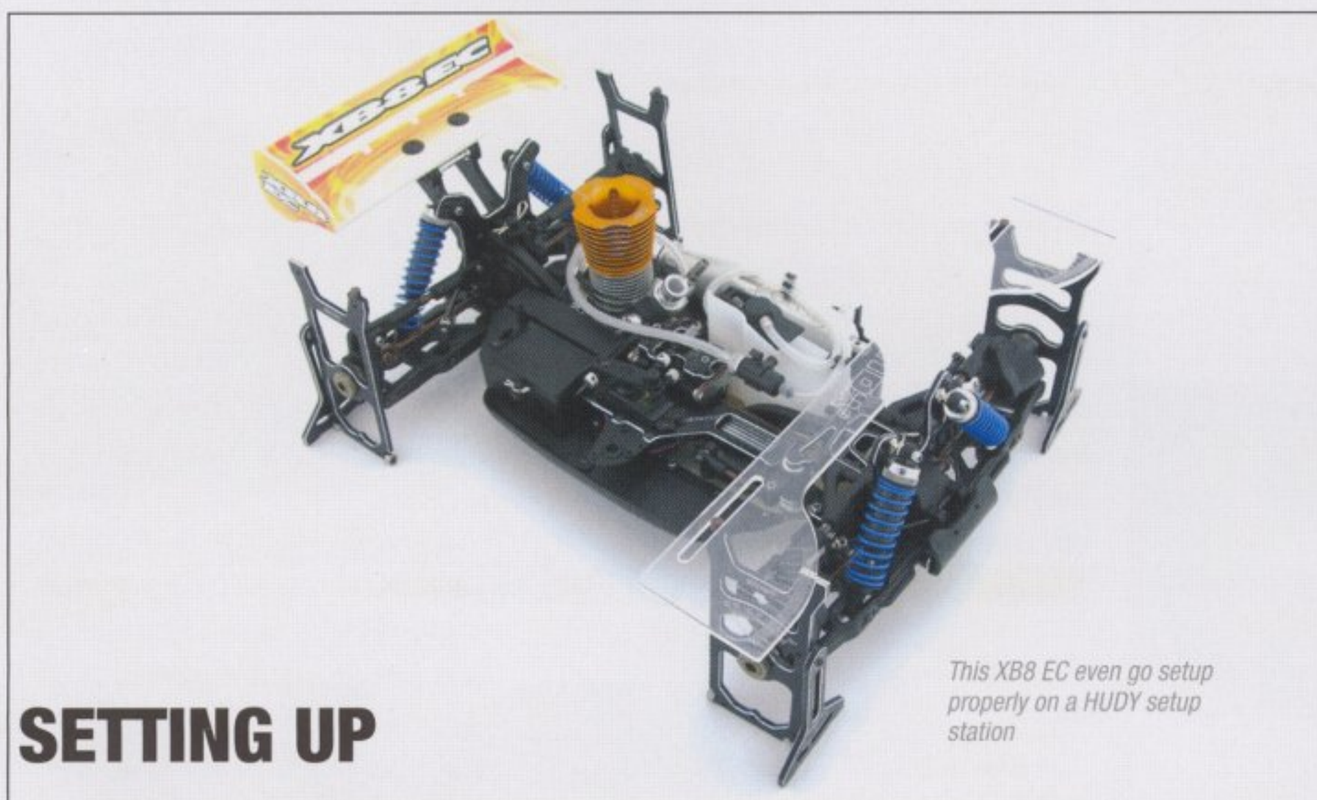
The fuel filter now attaches to the side of the 125cc fuel tank which reduces vibrations as it's mounted on rubber grommets
