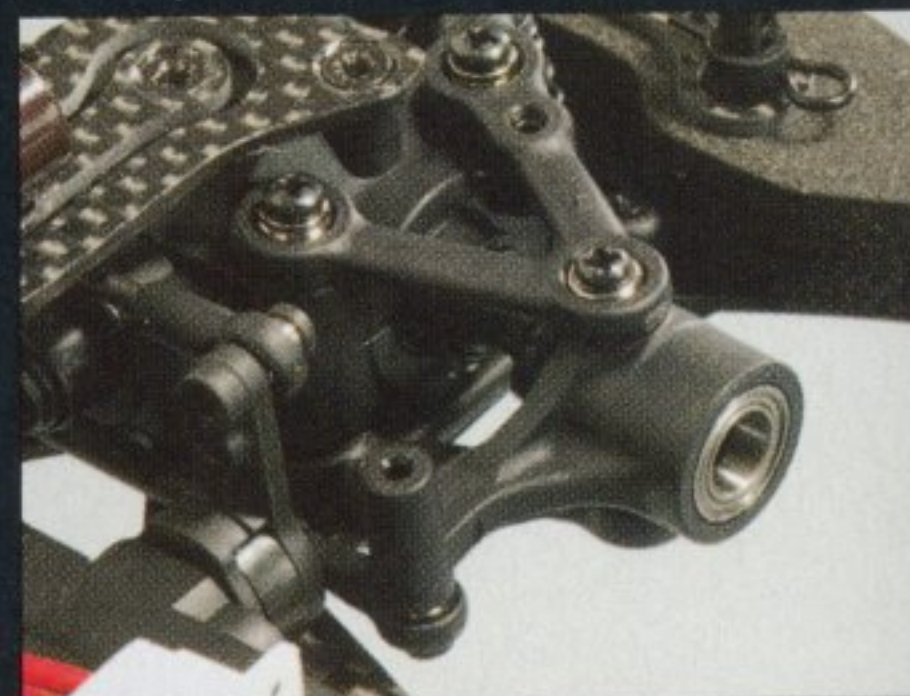
A strong servo-saver transfers motion to the steering knuckles. The two knuckles are linked by a long tie-rod. Ball bearings are seated in the hubs for the universal axles to spin on.
