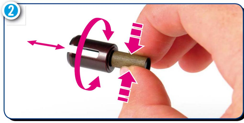
Roll the strip of sandpaper on the diff outdrive shaft, with the grit of the sandpaper against the shaft. Gently squeeze the sandpaper while turning the outdrive in both directions and moving it slightly in and out of the rolled sandpaper. Use a drop or two of light oil on the sandpaper (if desired) for smoother polishing. After finished polishing, carefully clean the diff outdrive to remove any residue or metal filings.
