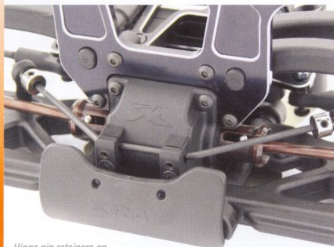
Hinge pin retainers on the front upper A-arms can be changed to alter the kick up and sway bars front and rear aid in the tuning
