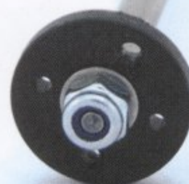
Two 1.5mm holes were added to the 1.3mm pistons to give an average of four 1.4mm holes
