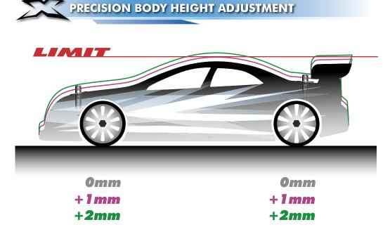
the T2 and NT1, while the body holders have the elevated mounting. This makes body height adjustment very easy and comfortable. In a few short seconds and clicks, you can exchange the body holders to adjust body height.
