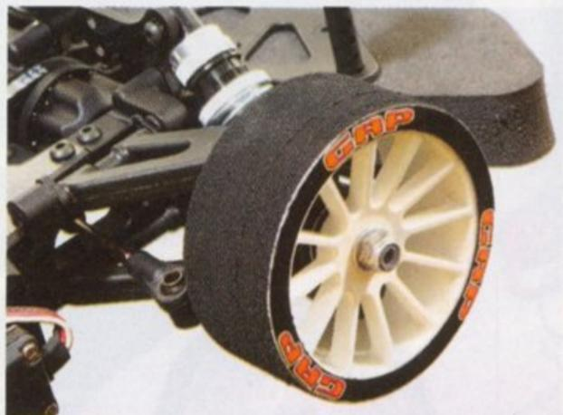
During our test, we used GRP tires. These tires are made from a high-quality foam material that provides excellent traction and wear.
