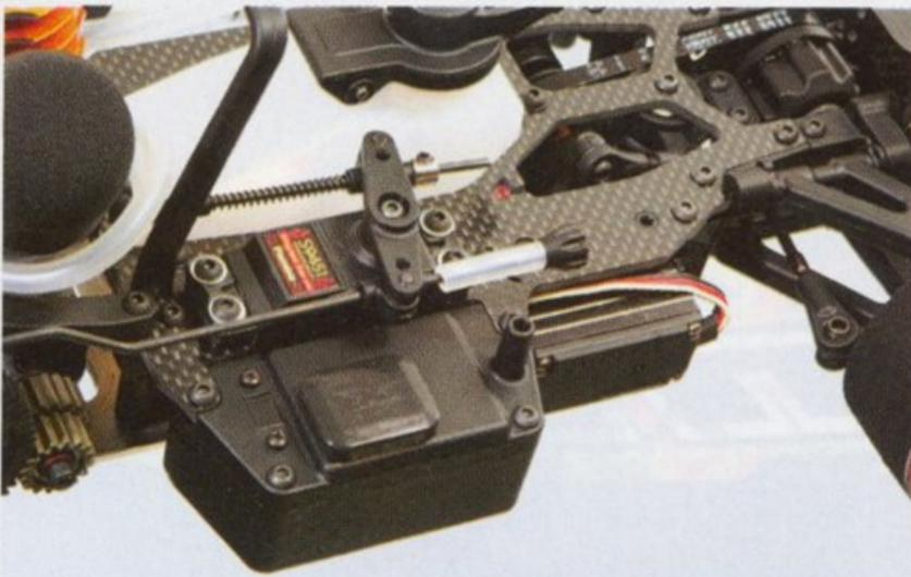
The radio box is completely sealed to protect your delicate radio equipment from dust and dirt. If a thin layer of silicone is added around the edge of the box, it becomes water-resistant.
