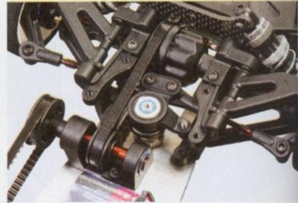
A center-mounted servo-saver rides on bearings to provide smooth operation. The servo-saver tension can be adjusted by the collar on the bottom of the post. Various Ackerman inserts are also included for maximum adjustments.
