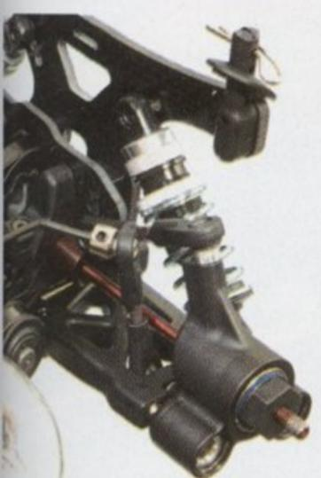
The rear assembly is similar to many of the 1/8 on-road cars on the market. The NT1 offers a beefy rear hub assembly to ensure maximum durability.
