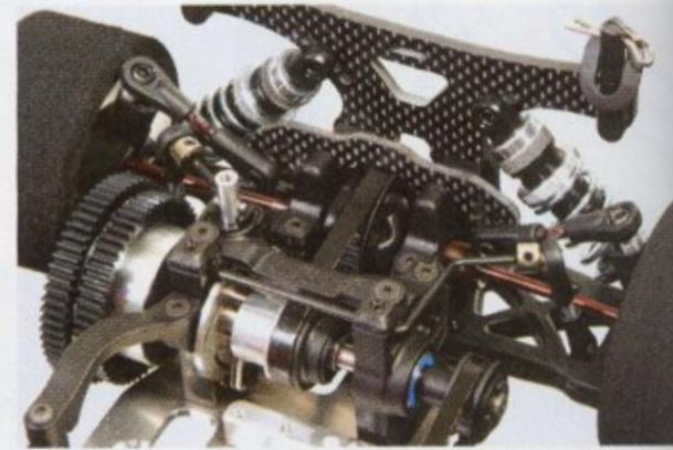
By removing just a few screws, the rear diff can be accessed easily to change the oil or to make belt-tension adjustments. A 2mm roll bar is standard to prevent chassis roll.
