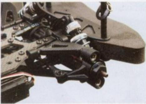
Camber and caster can be easily adjusted through clips and the pivot balls. Track width may also be adjusted through the pivot-ball front suspension.
