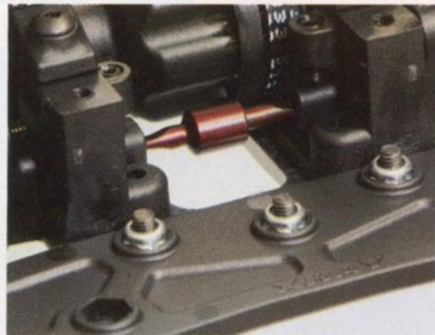
The front swaybar is fully adjustable. It allows quick adjustments on the fly during race day.
