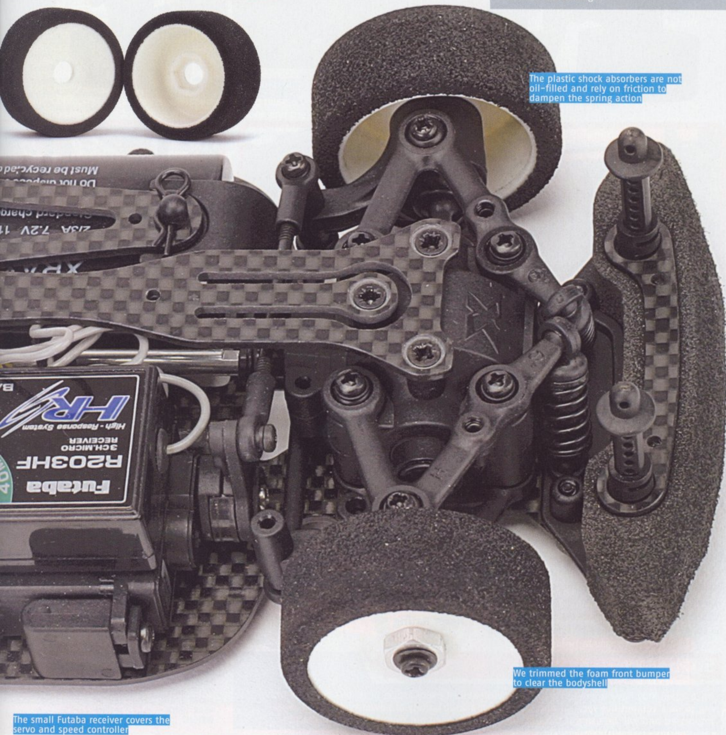
Above: The MFT upper chassis with slots to induce flex
