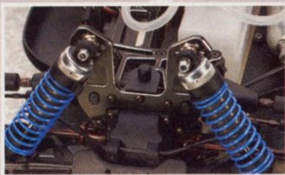
03 NICE CHASSIS • Swiss 7075 T6 aluminum is utilized in 3mm form to give the EC the strongest foundation possible. The XRAY engineers also took it upon themselves to redistribute the weight to bring it closer to the centerline to improve transitional handling. They also milled low-stress areas to make the chassis as light as possible without sacrificing durability.
