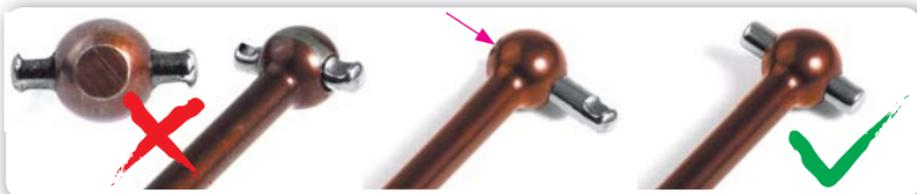
1 Do not use drive shafts when the pins are worn.
