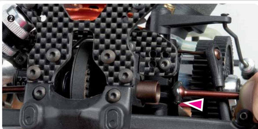
2 Insert the drive shaft into the outdrive and try to not remove the grease from the shaft.
