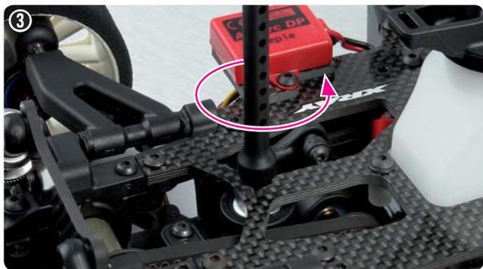
3 Screw the body post screw into the top of the servo saver. Tighten securely but be careful of stripping the plastic.
