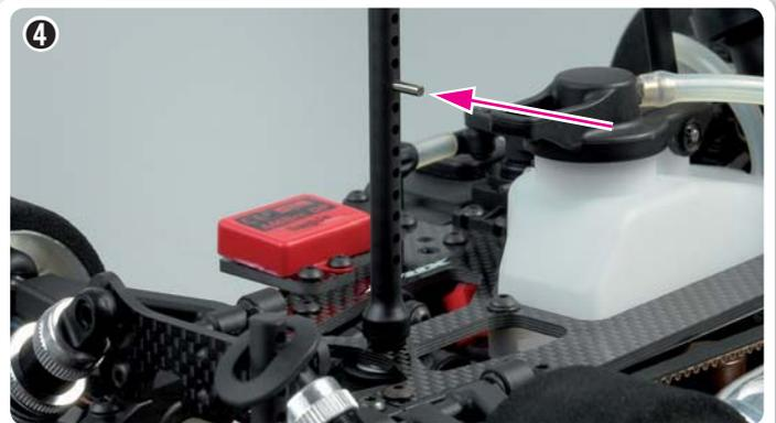
4 Find the best position for the mounting pin; the position depends on the body used. It is important to select a position that is BELOW the window.
