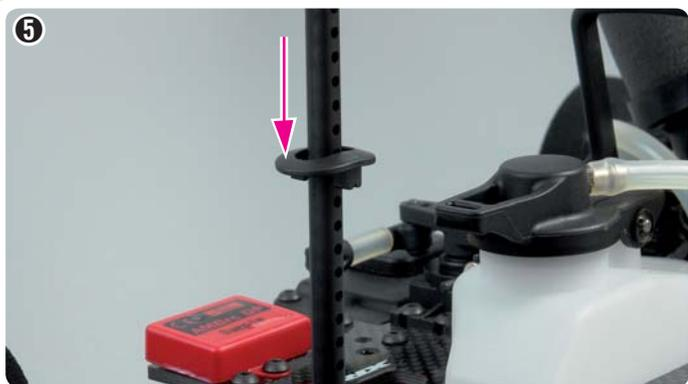
5 Press the body mount onto the pin until it snaps into place.
