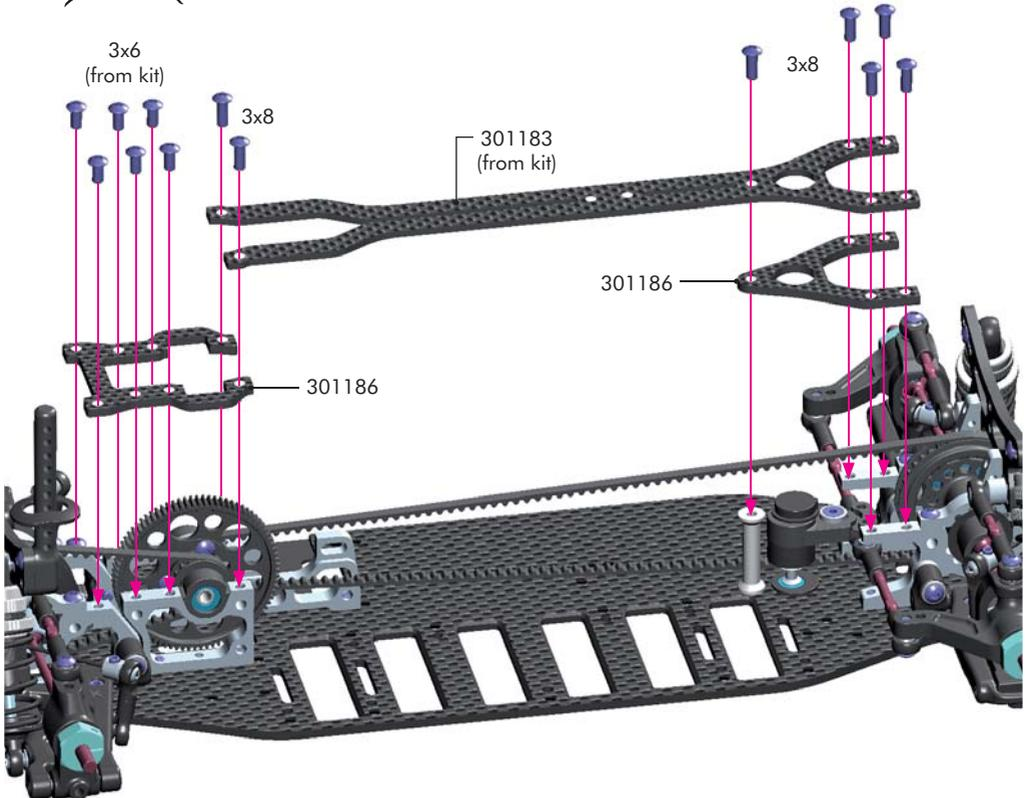
**NOTE!** The LiPo Conversion Set allows for the fitting of popular LiPo battery packs with a height of 24.5mm or less (the most popular and common configuration and sizing available on the market at the time of development). However, because of continuing development of LiPo batteries and no set of standardized regulations about battery sizes, XRAY cannot guarantee that all LiPo battery packs will fit in the EU Edition cars using this conversion set.
