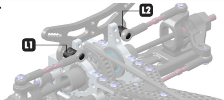
Using the 4.9mm roll-center holders in the front **makes the car turn easier and more precisely.**
