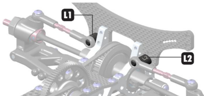
Using the 4.9mm roll-center holders in the rear **increases steering and stability.**
