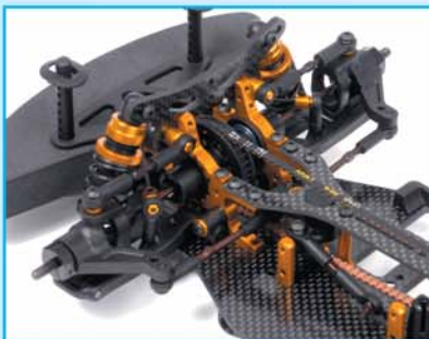
Servo saver positioned in absolute center of the chassis
