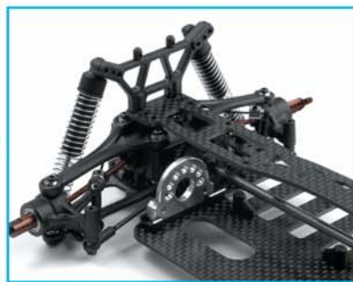
Ultra-efficient 4WD shaft drive system transfers all the power through the lightweight graphite center shaft
