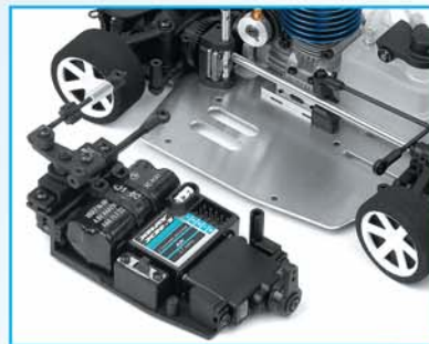
One-piece moulded radio tray allows easy quick access to radio equipment
