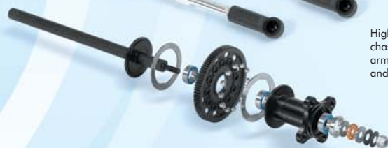
Super-lightweight rear axle features 1-piece high-grade precision hand ground graphite rod, precision carbide balls, hardened and ground D-steel shims, and premium carbide axial thrustbearing.
