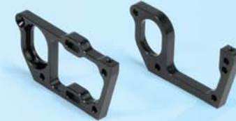
Ultra-light 7075 T6 Swiss CNC-machined bulkheads with integrated ride height adjustment
