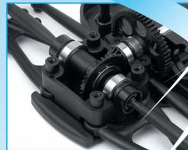
4WD shaft-drive transmission system
