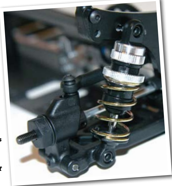
Shocks have hex drive ball mounts top and bottom so you simply unscrew, rather than pop them off
