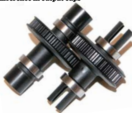
Front spool and rear diff, note the difference in output cups
