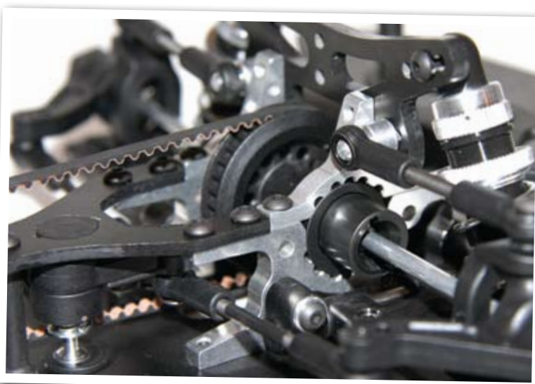
Front solid spool outputs
