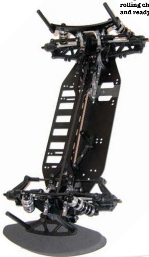
Xray T2R basic chassis with driveline assemblies installed
