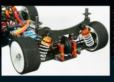
The T2009's rear shock tower is as low as possible to provide room for the body and also to keep weight low down.
