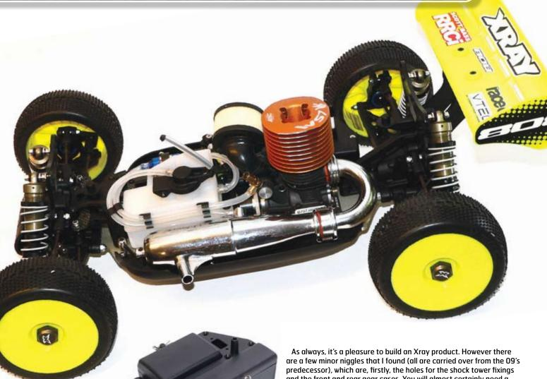
Above: Carbon radio tray with HB/HPI servos installed awaits attachment of PT and optional switch. We would prefer to see the battery box cover pinned on the opposite side Below: One of the few upgrades we fitted from the outset was the adjustable mount that enables engine swapping without having to realign the clutch bell and spur gear
