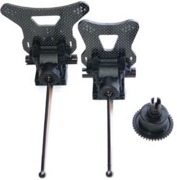
Above: Diff assembled ready to bolt on and you are soon looking at a rolling chassis
