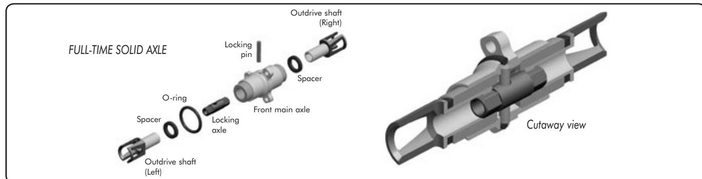
When using an XRAY Multi-Diff™ in “full-time solid axle” mode, both outdrive shafts (left and right) are connected to front main axle by internal locking axle and locking pin. The car achieves maximum 4WD braking, while being very stable and easy to drive.
