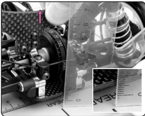
4. Keeping the ruler in place, slowly lift the chassis at its centerline. The chassis rises slightly until the wheels just lift from the set-up board.
