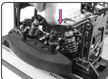
5. Push down and release the front and rear suspension a few times to settle it.
