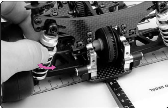
Spring preload is used primarily for adjusting ride height, and is not used for altering camber or other suspension settings or characteristics. Spring preload may also be used to adjust the tweak in the car. For more information, see sections "Ride Height" and "Tweak."
