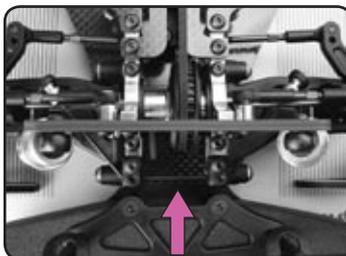
10. Attach the front anti-roll bar.
