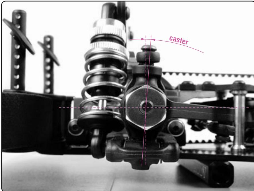
Caster describes the forward/backward angle of the front steering block with respect to a line perpendicular to the ground. Caster angle affects on- and off-power steering, as it tilts the chassis more or less depending on how much caster is set. Generally, a lower caster angle (more upright) is better on slippery, inconsistent, and rough surfaces, and a higher caster angle (more inclined) is better on smooth, high-traction surfaces.
