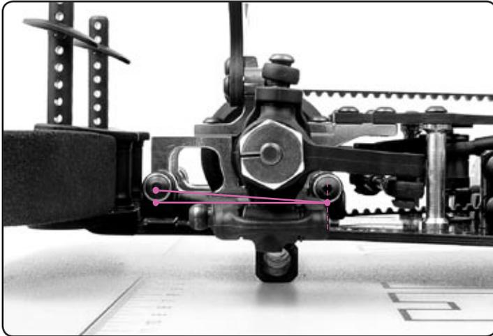
Front anti-dive is used as a tuning aid to run a softer front spring rate without introducing a tendency to dive downward too much in the front under braking. In order to prevent 100% of the cars weight transfer force from being exerted onto the softer springs anti-dive is used to allow a certain percentage of the weight transfer to be absorbed by the front lower arms.
