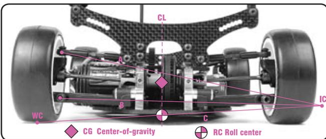
Roll center is determined by the car’s suspension geometry. Each end of the car has its own roll center, determined by the suspension geometry at that end of the car.
