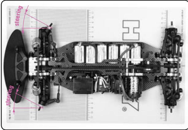
Although most cars' front suspension geometry is designed such that the turning radius of the car is the same from left to right, sometimes this isn't the case. You can use the toe gauge plate to make sure that the steering turns as sharply to the left as it does to the right.
