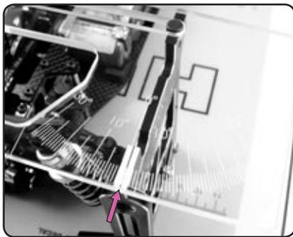
To read the toe value of the right rear wheel, push the toe gauge to the left until the pin on the top edge of the right set-up stand hits the edge of the slot in the toe gauge. Read the measurement.
