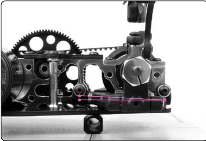
Rear anti-squat is used as a tuning aid primarily when cars need to run a soft rear spring rate and they have a tendency for the rear end to squat down too much under acceleration. An added benefit of anti-squat is quicker initial acceleration at the start of a race. In order to prevent 100% of the car's weight transfer force from being exerted onto the softer springs, anti-squat is used to allow a certain percentage of the weight transfer to be absorbed by the rear lower arm motion.
