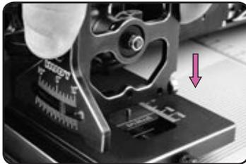
4. Mount the FRONT set-up stands on the tweak station pins. Place the REAR set-up stands on the set-up board. (You do this to check for tweak at the REAR of the car).
