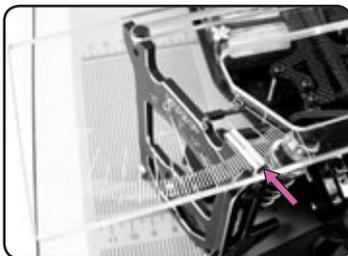
7. Push the toe gauge to the right until the pin on the top edge of the left set-up stand hits the edge of the slot in the toe gauge.
