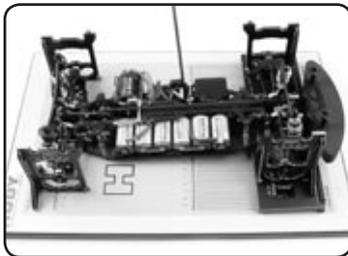
**NOTE:** It is very important that the car has symmetrical track-width at front and rear. For more information, see “Track-Width” section.
