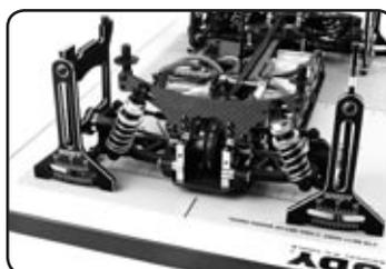
5. Read the camber setting from the camber gauge of each of the four set-up stands.
