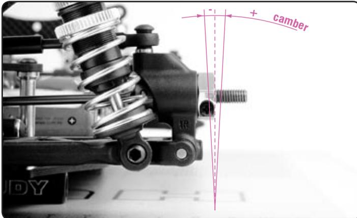
Camber is the angle of a wheel to the surface on which the car is resting (with wheels and shock absorbers mounted). Zero degrees ( $0^\circ$ ) of camber means that the wheel is perpendicular to the reference surface. Negative camber means that the top of the wheel is leaning inwards towards the centerline of the car. Positive camber means that the top of the wheel is leaning outwards from the centerline of the car. Camber affects the car's side traction.
