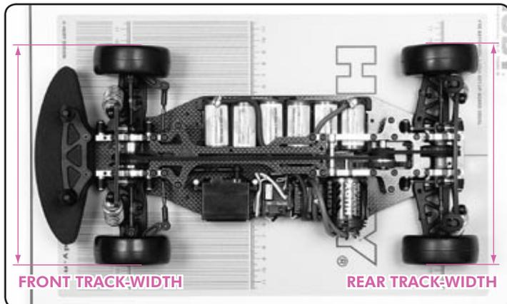
Track-width is the distance between the outside edges of the wheels, front or rear, and it affects the car's handling and steering response. It is important that front or rear track-width is adjusted symmetrically, meaning that the left and right wheels must be the same distance from the centerline of the chassis.
