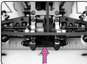
9. Attach the rear anti-roll bar.
