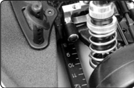
3. Measure the ride height using the ride height gauge at the front and rear of the car at the lowest points of the chassis.
