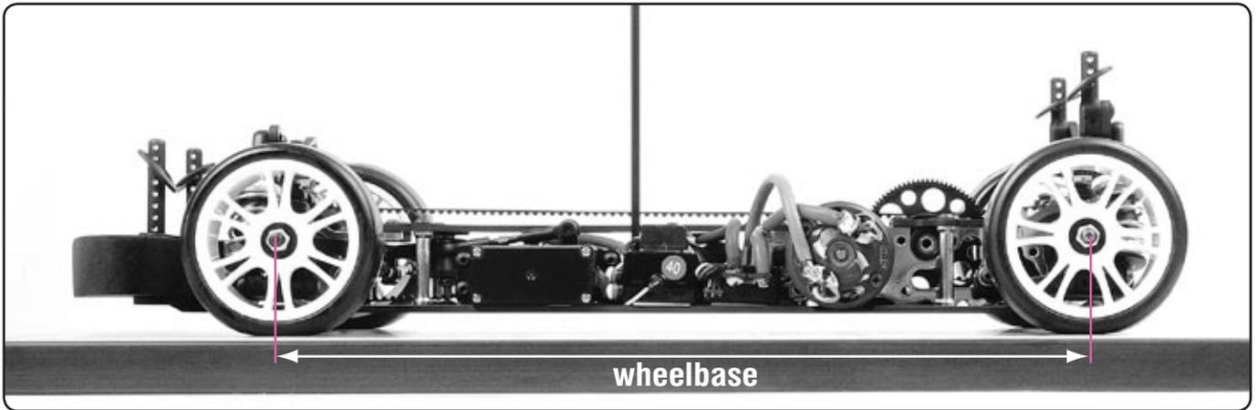
Wheelbase refers to the horizontal distance between the front and rear axles. Changes to wheelbase can have a dramatic effect on the handling of your car, since it readjusts the distribution of weight on the wheels, which adjusts traction. Not all R/C cars have the option to adjust the wheelbase.
