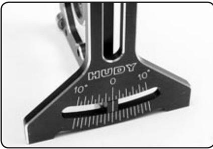
Each graduated mark indicates a 1° camber value. You should be able to set camber with a resolution of 0.5°
