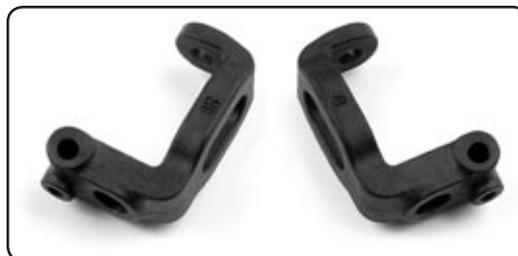
Note that depending on the track surface and tire hardness, these effects may be different in that you may always have more steering with more caster. This is especially true for high-traction tracks and/or soft tires.
