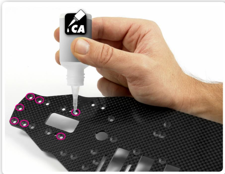
We strongly recommend that you apply CA glue to the countersunk holes in the chassis where the front aluminum arm holders are mounted. Apply a small drop of CA glue to each countersunk hole and spread the glue around the countersunk surface; this will help to strengthen the hole and prevent damage from a hard crash.
