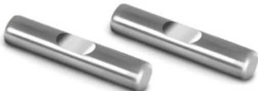
To help prevent loosening of the setscrew from the CVD shaft, XRAY recommends using these new pins with flat spots. The flat spots allow the setscrew to better settle into the coupling.
