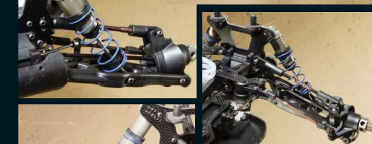
The front end is made up of adjustable upper camber links, lightweight outdrives, lightened hubs, and carbon fiber tower and top plate.
