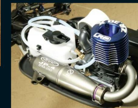
One major update to the XT8 '09 is the addition of the extended motor mounts, eliminating the unwanted chassis flex of the original XT8. The LRP .30 is an awesome mill for practice or for you backyard bashers, but for racing you'll probably want a .21.
