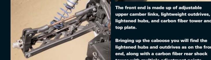
Bringing up the caboose you will find the lightened hubs and outdrives as on the front end, along with a carbon fiber rear shock tower with multiple adjustment points.
