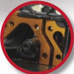
Bulkhead and layshaft mounts are separate
