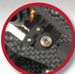
Centre point steering allows fine tuning of the geometry
