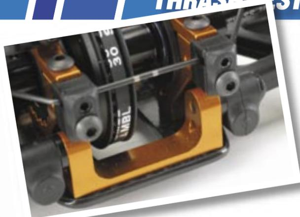
Orange alloy brace at the rear connects the two suspension mounts
