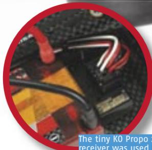
The tiny KO Propo 2.4GHz receiver was used
