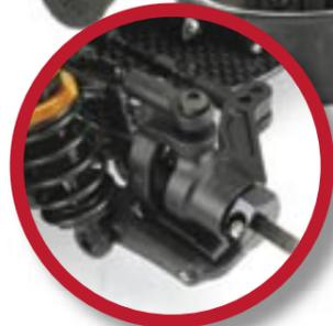
Pinch bolt system secures the wheel hex to the axle
