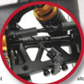
Alloy driveshafts, drop screws and optional anti-roll bar mountings
