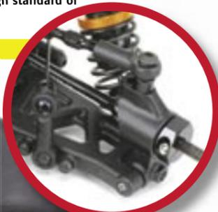
Design uses a grub screw to secure the hinge pin
