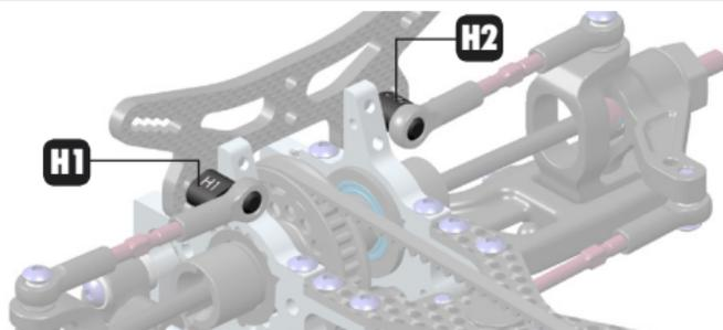
Using the H roll-center holders in the front makes the car turn easier. Recommended for high-traction carpet tracks because it decreases corner steering and help prevent traction rolling.
