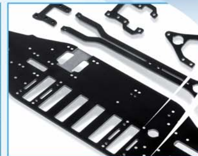
Fiberglass chassis, top deck and shock towers
