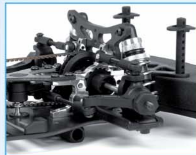
Lowest ultra-lightweight Swiss 7075 T6 bulkheads
