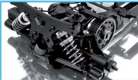
CNC-machined 3mm Swiss 7075 T6 chassis
