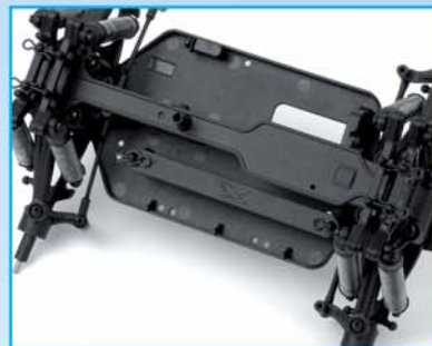
Fully-independent suspension front & rear
