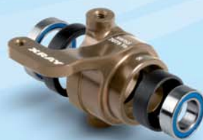
#352256 XB808 Alu Steering Block Right - Swiss 7075 T6 - Hard Coated
