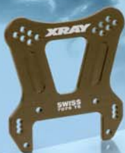
#352093 XB808 Front Alu Shock Tower Swiss 7075 T6 (3mm) - Hard Coated
