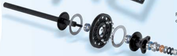
Super-lightweight rear axle features 1-piece high-grade precision hand ground graphite rod, precision carbide balls, hardened and ground D-steel shims, and premium carbide axial thrustbearing.
