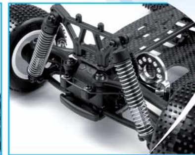
Adjustable shock positions front & rear
