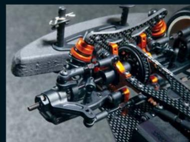
Above: to lower the chassis' center of gravity the new T3 has significantly shorter shocks and towers to match. Left: redesigned steering blocks give you more directional control.
