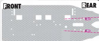
The rear aluminum holders have integrated rear toe-in (approximately 1° rear toe-in).
