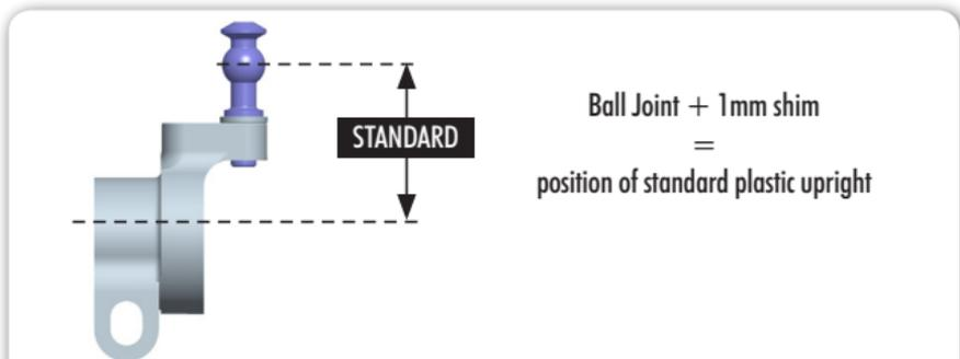
By adding or removing shims under the ball, upper roll center position is changing.
