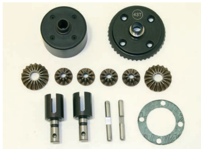
Above: One of the three diff's stripped out for all to see
