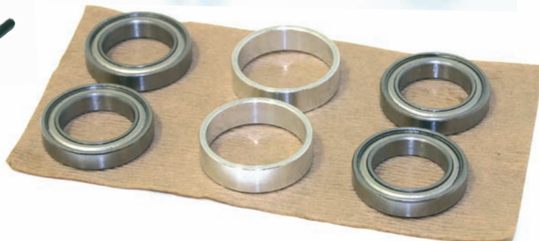
Above: The diff pinion bearings are a new size with a spacing collar
