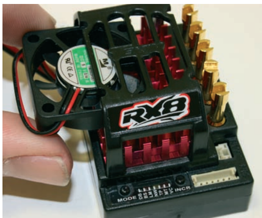
Above: The Tekin RX8 speed control comes with a huge cooling fan that needs fitting before use
