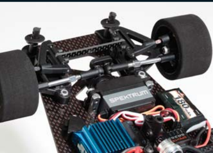
The Spektrum steering servo has a cool looking aluminum mid-section that keeps the servo cool during operation. The steering servo is mounted flat to the chassis to give the XII a low CG. Xray does include spacers to adjust the servo location depending on the brand of servo you choose.
