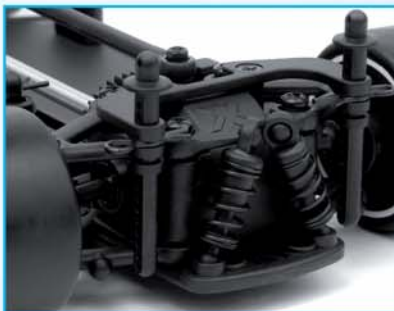
Adjustable shock positions front & rear
