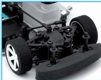
Fully-independent front suspension for precise and responsive handling
