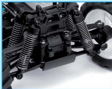
Fully-independent suspension front & rear for precise and responsive handling
