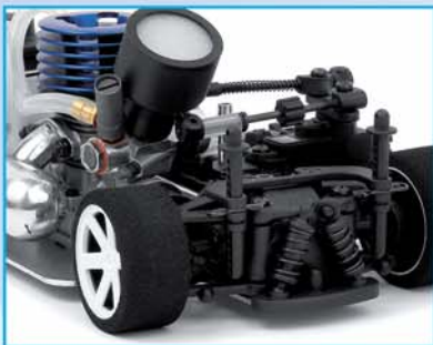
Fully-independent rear suspension
