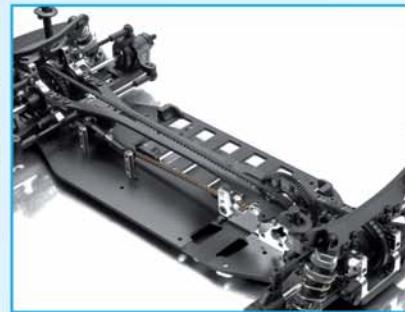
Fibre chassis, top deck and shock towers
