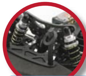
Fibreglass is used for the chassis, top deck and shock mounts
