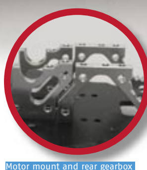
Motor mount and rear gearbox housing are separate items
