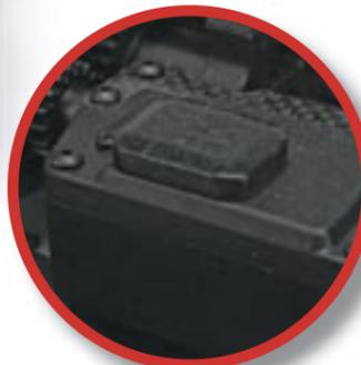
A neat rubber access bung allows access to the receiver
