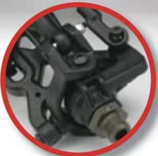
Although this set-up looks all plastic, there are inserts in the steering arms for the king pins to screw into
