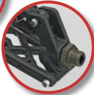
Like its nitro relative, the rear hubs are secured by hinge pins with nuts for security
