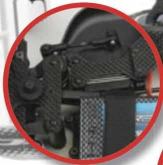
Carbon fibre is used for the towers, radio tray and more
