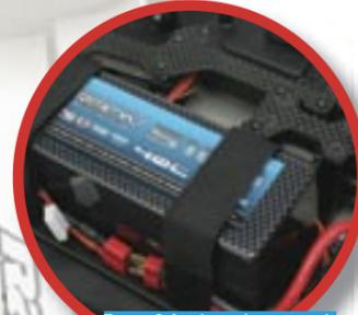
Team Orion's carbon cased 14.8V 5100mAh 40C LiPo
