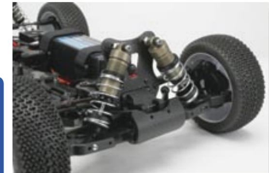
Note the use of different allen bolts on the lower shock fixing to prevent them from un-doing on track
