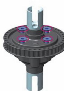
Tighten the screws equally but do NOT tighten them completely.
